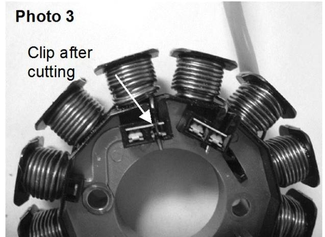
3. Once the clip has been cut, grab the wire with a pair of needle nose pliers and carefully bend it up out of the clip slot. Use a sharp blade to scrape the layer of brown enamel coating from the last  $\frac{1}{4}$ " of the wire to expose shiny bare copper. See Photo 4.
