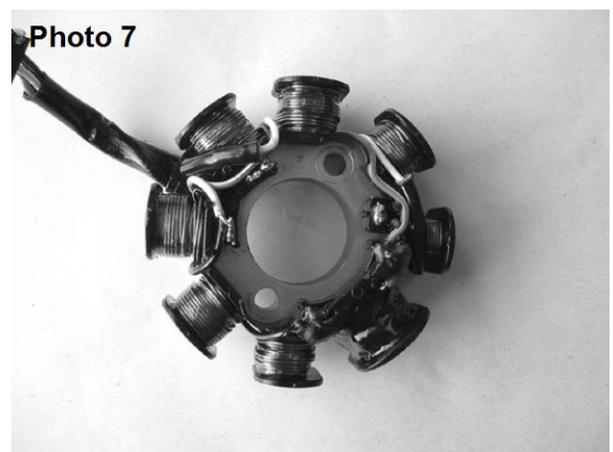
The modification is now complete. Before reinstalling the stator you can check your work by verifying with an Ohmmeter that the yellow and white wires from the stator have continuity only with each other and not with the metal body of the stator. There should be very low resistance (approximately .5 Ohm) between the yellow and white wires. If it looks good, go ahead and reinstall the stator onto the motorcycle.
