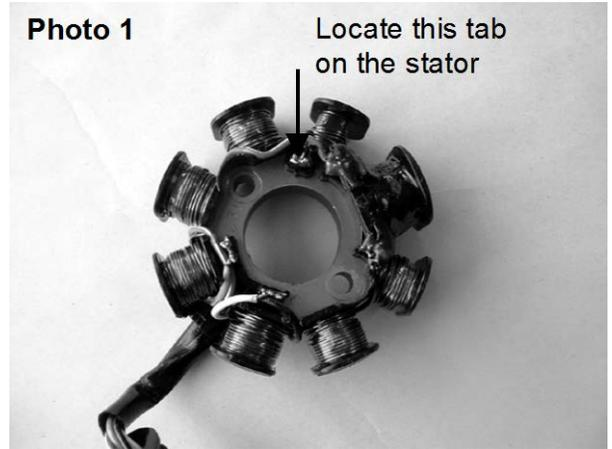
2. Using a soldering iron, melt the solder and push up on the copper wire at the same time to release it from the tab. Try not to bend the copper wire sharply as this will weaken it and cause it to break. You can temporarily move the red/white wire from its guide to allow the unsoldered copper wire to pass under it easier. See Photo 2.
